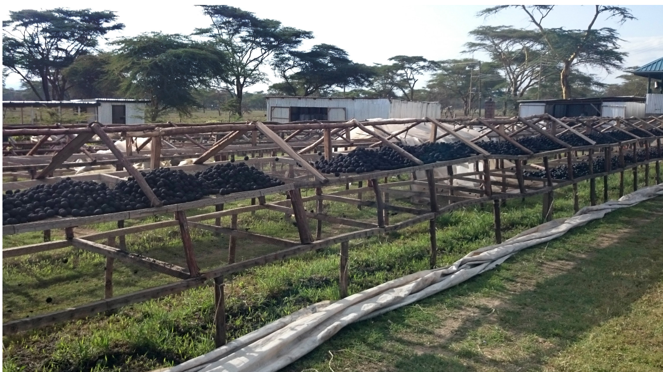
Charcoal briquettes derived from waste drying at the Sanivation treatment site.
